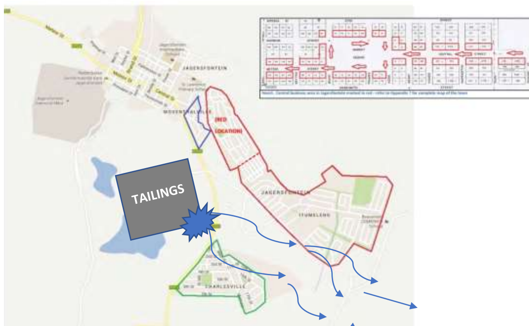
Figure 4 Breach and direction of the flow of the slurry on the impacted sections of Charlesville and Itumeleng (Adapted from Philip, 2014)
